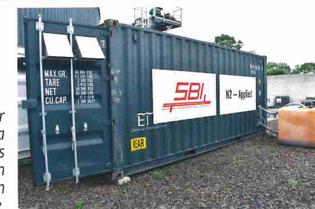
The plasma reactor is housed in a container and directs the liquid nitrogen into a IBC collection tank for storage.
